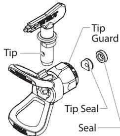
**NOTE: The arrow on the tip handle should be pointing in the forward direction for spraying.**
