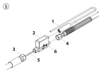
**7.** At the heater block, remove the four screws that secure the hose heater cover (Fig. 6, item 1).
