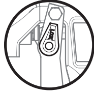
Trigger unlocked (gun will spray)
