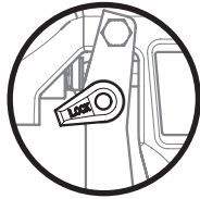
Trigger locked (gun will not spray)
