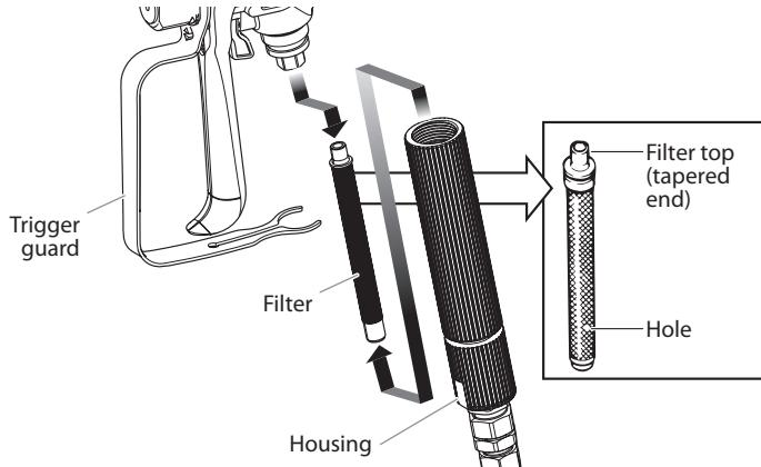
2. Remove the filter from the spray gun housing and clean with the appropriate cleaning solution (warm, soapy water for latex paints, mineral spirits for oil-based materials).
