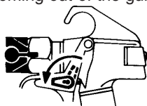
Trigger lock in locked position.
