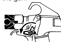
Trigger lock in locked position.
