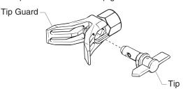
2. Thread the tip guard onto the gun. Position the tip guard in the desired spraying position, then tighten securely by hand.
