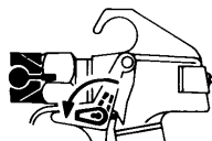
Trigger lock in locked position.
