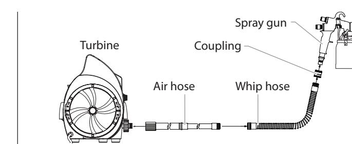
**IMPORTANT:** Do not attach the short air whip hose directly to the turbine, as the hose will become damaged.
