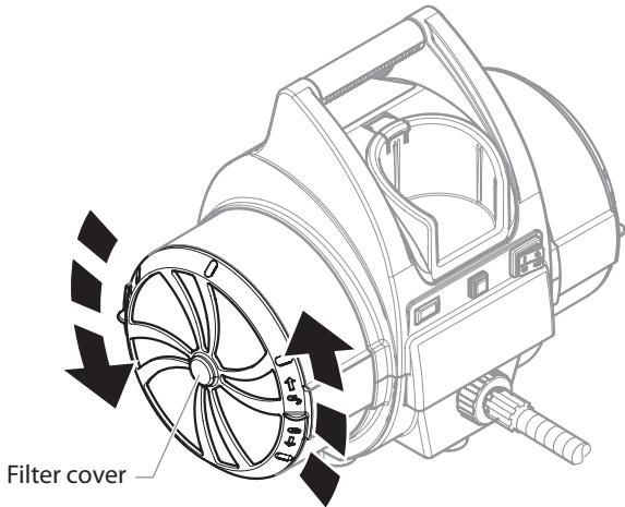
2. Remove each filter set (pre-filter and filter) from the filter housing on each side of the turbine.
