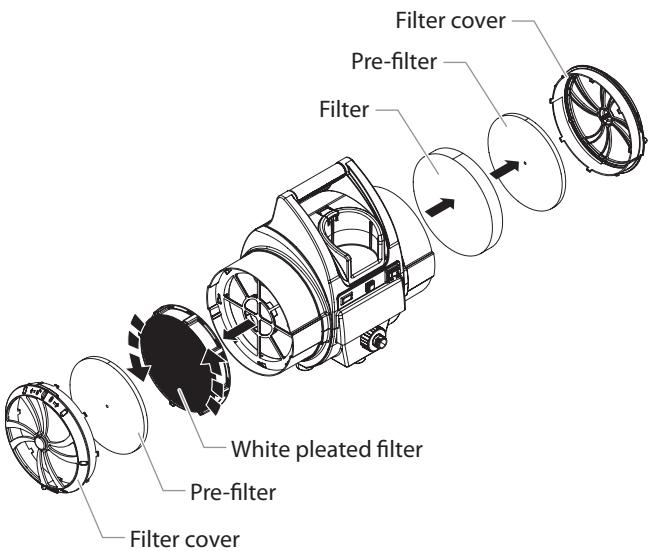
3. Clean the filters. Either tap the filters to knock out the contaminants or use pressurized air to blow out the contaminants. For material that is not blown or knocked loose easily, soak the filters in soapy water or mineral spirits. Allow the filters to dry completely before placing them back in the turbine.
