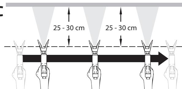
**If very sharp edges result or if there are streaks in the spray jet – increase the operating pressure or dilute the coating material.**
