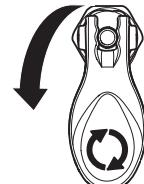
6. Set the pressure to RAPID CLEAN by turning the pressure control knob to its RAPID CLEAN position.
