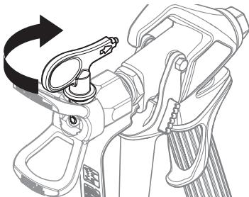
3. Flip the PRIME/SPRAY valve lever to the SPRAY position.
